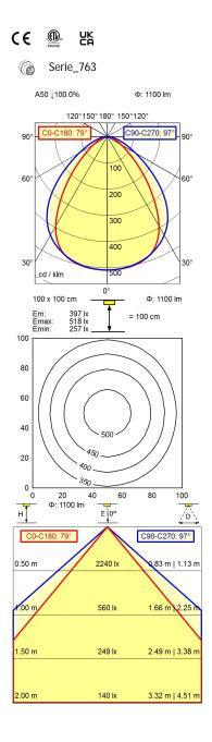
Light source LED Work equipment Without **Connected load** 18 - 30 V; DC **Power consumption** ca. 12 W Luminous flux approx. 1.100 lm Luminous efficiency approx. 91 lm/W Light type/-color Cold white Colour temperatur approx. 5.000 K Color rendering index CRI ≥ 80
