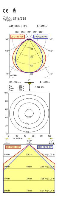
Light sourceLEDWork equipmentWithoutConnected load22 - 26 V; DCPower consumptionca. 19 W
