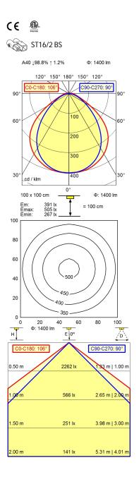
Light sourceLEDWork equipmentWithoutConnected load22 - 26 V; DCPower consumptionca. 19 W
