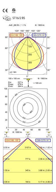
Light source LED Work equipment Without **Connected load** 22 - 26 V; DC ca. 25 W **Power consumption**
