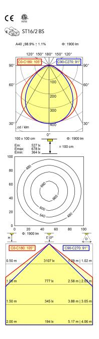
Light sourceLEDWork equipmentWithoutConnected load22 - 26 V; DCPower consumptionca. 25 W
