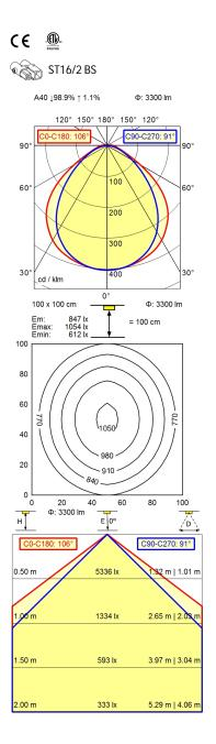
Light source LED Work equipment Without **Connected load** 22 - 26 V; DC **Power consumption** ca. 44 W
