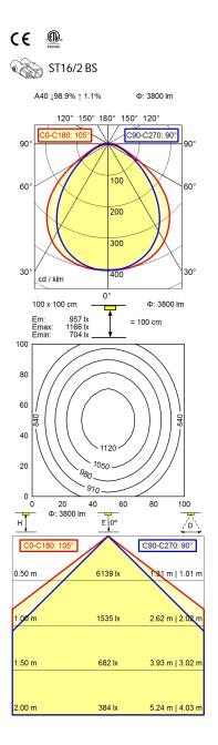
Light sourceLEDWork equipmentWithoutConnected load22 - 26 V; DCPower consumptionca. 50 W
