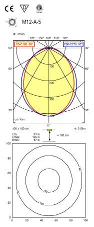
Light source LED Work equipment Without Connected load 22 - 26 V; DC ca. 3 W **Power consumption** Luminous flux approx. 315 lm Cold white Light type/-color Colour temperatur approx. 5.000 K Color rendering index CRI ≥ 80 **Light distribution** Direct 89° / 97° Beam angle **Chromaticity tolerance LED** < 4 SDCM Glare control Screen System of protection IP 54
