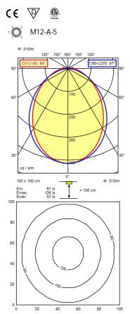
Light source LED Work equipment Without **Connected load** 22 - 26 V; DC **Power consumption** ca. 3 W Luminous flux approx. 315 lm Cold white Light type/-color Colour temperatur approx. 5.000 K Color rendering index CRI ≥ 80 Light distribution Direct Beam angle 89° / 97° **Chromaticity tolerance LED** < 4 SDCM Glare control Screen System of protection IP 54
