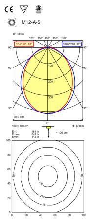
Light source LED Work equipment Without **Connected load** 22 - 26 V; DC **Power consumption** ca. 6 W Luminous flux approx. 630 lm Cold white Light type/-color Colour temperatur approx. 5.000 K Color rendering index CRI ≥ 80 Direct
