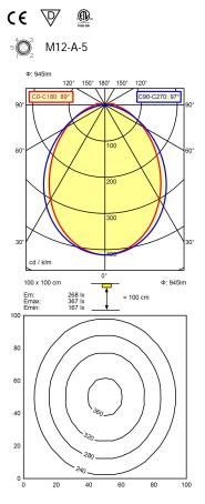
Light source LED Work equipment Without Connected load 22 - 26 V; DC ca. 9 W **Power consumption** approx. 945 lm Luminous flux Cold white Light type/-color Colour temperatur approx. 5.000 K Color rendering index CRI ≥ 80 **Light distribution** Direct 89° / 97° Beam angle **Chromaticity tolerance LED** < 4 SDCM Glare control Screen System of protection IP 54 Class of protection Ш
