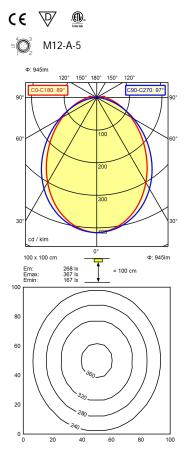
Light source LED Work equipment Without **Connected load** 22 - 26 V; DC ca. 9 W **Power consumption** approx. 945 lm Luminous flux Cold white Light type/-color Colour temperatur approx. 5.000 K Color rendering index CRI ≥ 80 **Light distribution** Direct 89° / 97° Beam angle **Chromaticity tolerance LED** < 4 SDCM Glare control Screen System of protection IP 54
