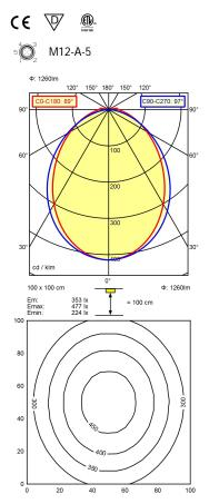
Light source LED Work equipment Without Connected load 22 - 26 V; DC ca. 12 W **Power consumption** Luminous flux approx. 1.260 lm Cold white Light type/-color Colour temperatur approx. 5.000 K Color rendering index CRI ≥ 80 **Light distribution** Direct 89° / 97° Beam angle **Chromaticity tolerance LED** < 4 SDCM Glare control Screen System of protection IP 54 Class of protection Ш
