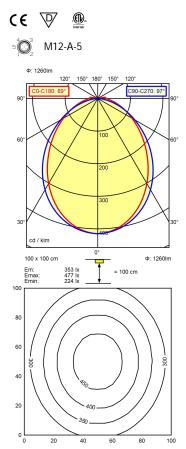
Light source LED Work equipment Without Connected load 22 - 26 V; DC **Power consumption** ca. 12 W Luminous flux approx. 1.260 lm Cold white Light type/-color Colour temperatur approx. 5.000 K Color rendering index CRI ≥ 80 **Light distribution** Direct Beam angle 89° / 97° **Chromaticity tolerance LED** < 4 SDCM
