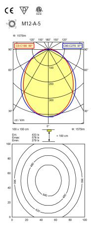
Light source LED Work equipment Without **Connected load** 22 - 26 V; DC ca. 15 W **Power consumption** Luminous flux approx. 1.575 lm Cold white Light type/-color Colour temperatur approx. 5.000 K Color rendering index CRI ≥ 80 Direct **Light distribution** 89° / 97° Beam angle **Chromaticity tolerance LED** < 4 SDCM Glare control Screen
