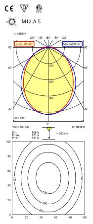
Light source LED Work equipment Without Connected load 22 - 26 V; DC ca. 18 W **Power consumption** Luminous flux approx. 1.890 lm Cold white Light type/-color Colour temperatur approx. 5.000 K Color rendering index CRI ≥ 80 **Light distribution** Direct 89° / 97° Beam angle **Chromaticity tolerance LED** < 4 SDCM Glare control Screen System of protection IP 54
