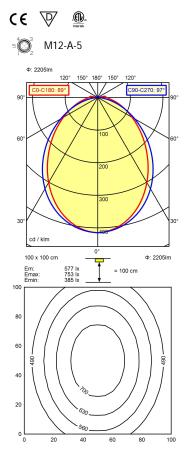
Light source LED Work equipment Without **Connected load** 22 - 26 V; DC ca. 21 W **Power consumption** Luminous flux approx. 2.205 lm Cold white Light type/-color Colour temperatur approx. 5.000 K Color rendering index CRI ≥ 80 Light distribution Direct 89° / 97° Beam angle **Chromaticity tolerance LED** < 4 SDCM Glare control Screen
