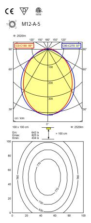
Light source LED Work equipment Without Connected load 22 - 26 V; DC ca. 24 W **Power consumption** Luminous flux approx. 2.520 lm Cold white Light type/-color Colour temperatur approx. 5.000 K Color rendering index CRI ≥ 80 **Light distribution** Direct 89° / 97° Beam angle **Chromaticity tolerance LED** < 4 SDCM Glare control Screen
