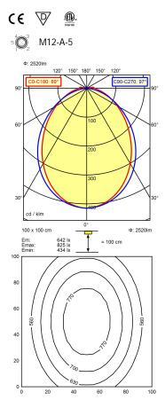
Light source LED Work equipment Without Connected load 22 - 26 V; DC ca. 24 W **Power consumption** Luminous flux approx. 2.520 lm Cold white Light type/-color Colour temperatur approx. 5.000 K Color rendering index CRI ≥ 80 **Light distribution** Direct 89° / 97° Beam angle **Chromaticity tolerance LED** < 4 SDCM Glare control Screen System of protection IP 54
