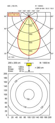
Light source LED Work equipment Electronic ballast **Connected load** 220 - 240 V; 50 Hz; 60 Hz **Power consumption** ca. 14 W Standby ca. 0,2 W
