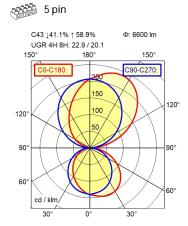
work equipment electronic ballast dimable digital connected load 220 - 240 V; AC; 50 Hz; 60 Hz power consumption ca. 50 W luminous flux approx. 6.600 lm luminous efficiency approx. 132 lm/W light type/-color adjustable white colour temperatur approx. 3.000 - 6.500 K color rendering index CRI ≥ 80 light distribution direct/indirect direct ratio approx. 41 %
