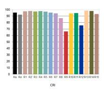
Work equipment Power supply unit **Connected load** 220 - 240 V; 50 Hz; 60 Hz **Power consumption** ca. 85 W Luminous flux approx. 10.200 lm Luminous efficiency 1) approx. 120 lm/W Light type/-color Cold white Colour temperatur approx. 4.000 K Color rendering index  $CRI \ge 90; R9 \ge 50$ Light distribution Direct/indirect **Direct ratio** approx. 50 % Glare control optical film Luminance (L65)  $\leq 2.600 \text{ cd/m}^2$ Unified glare rating (4H 8H) 2 ≤ 16
