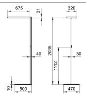
Work equipment Electronic ballast **Connected load** 220 - 240 V; AC; 50 Hz; 60 Hz **Power consumption** ca. 90 W Luminous flux approx. 15.000 lm Luminous efficiency 1) approx. 166 lm/W Light type/-color Cold white Colour temperatur approx. 4.000 K Color rendering index CRI ≥ 90: R9 ≥ 50 Light distribution Direct/indirect **Chromaticity tolerance LED** < 3 SDCM Glare control Prism aperture Luminance (L65)  $\leq 3.000 \text{ cd/m}^2$ UGR class (4H 8H; EN 12464-1) ≤ 16
