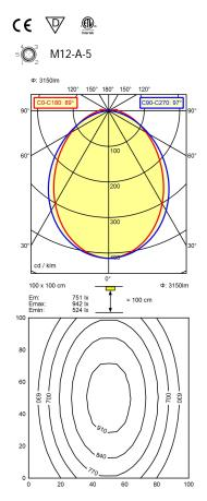
Light source LED Work equipment Without **Connected load** 22 - 26 V; DC ca. 30 W **Power consumption** Luminous flux approx. 3.150 lm Cold white Light type/-color Colour temperatur approx. 5.000 K Color rendering index CRI ≥ 80 Light distribution Direct 89° / 97° Beam angle **Chromaticity tolerance LED** < 4 SDCM
